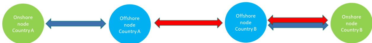
Figure 23 Case 2.1 – Project between two offshore nodes and expansion of one radial connection ENTSO-E | Rue de Spa, 8 | 1000 Brussels | info@entsoe.eu | www.entsoe.eu | @entso_e
