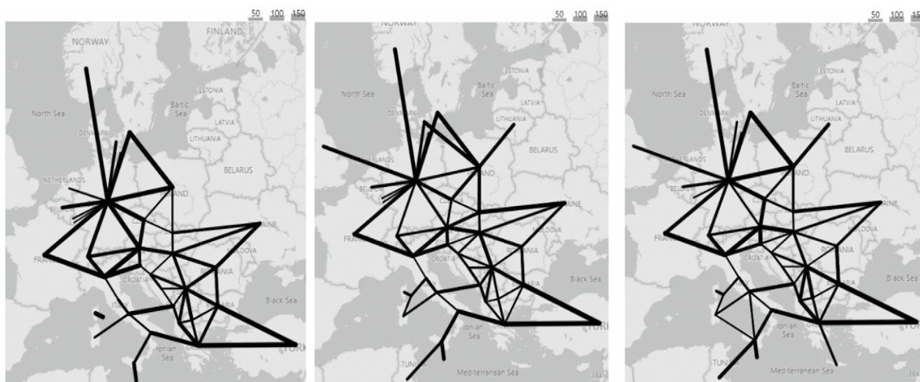
Figure 6 – Percentage of hours per year where the flow of electricity reaches 100 % of the Net Transfer Capacity on the border (constraint duration), in No investment after 2020 (left), SEW-based needs (middle) and Portfolio 2030 (right)
