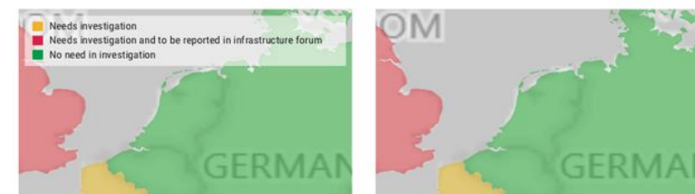
Figure 6.2: Ratio of nominal transmission capacity to the peak load in 2030, in the situation where Europe would stop investing in the grid after 2020 (left) and in the expected grid in 2025 (right).
