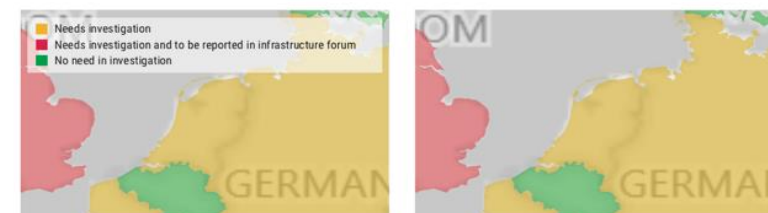
Figure 6.2: Ratio of nominal transmission capacity to the peak load in 2030, in the situation where Europe would stop investing in the grid after 2020 (left) and in the expected grid in 2025 (right).
