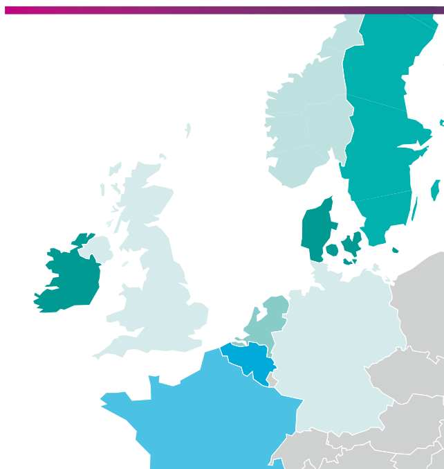
Figure 15 – This map shows per country whether the annual onshore and offshore RES production exceeds or falls short to the annual demand. Green indicates it exceeds and blue it falls short. Note: offshore wind from the Northern Seas is taken into account only in this analysis.
