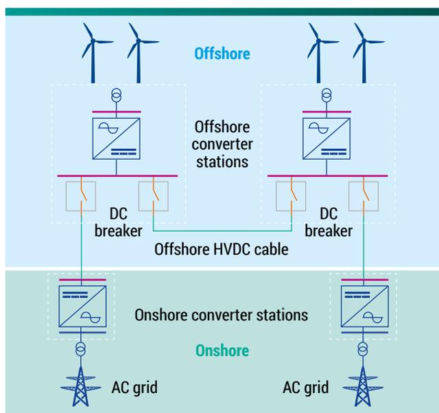
Figure 11 – Example of a hybrid configuration using DC breakers, with only one converter per offshore substation, and DC breakers protecting the HVDC links.
