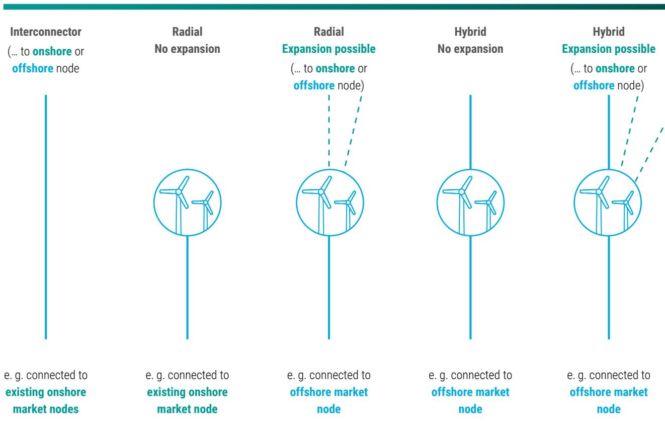
Figure 8 – Representation of node-connection-options (to be specified by the RGs).
