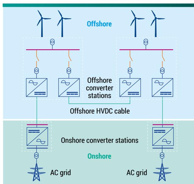
Figure 12 – Example of a hybrid configuration without using DC breakers, with one converter per each HVDC link.
