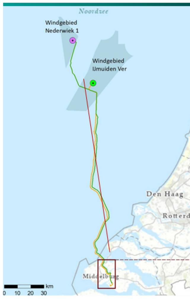
Figure 17 – Cable route of OWF Nederwiek VS straight point-to-point line, an example of the adaptations considered in the 15 % addition mentioned above.
