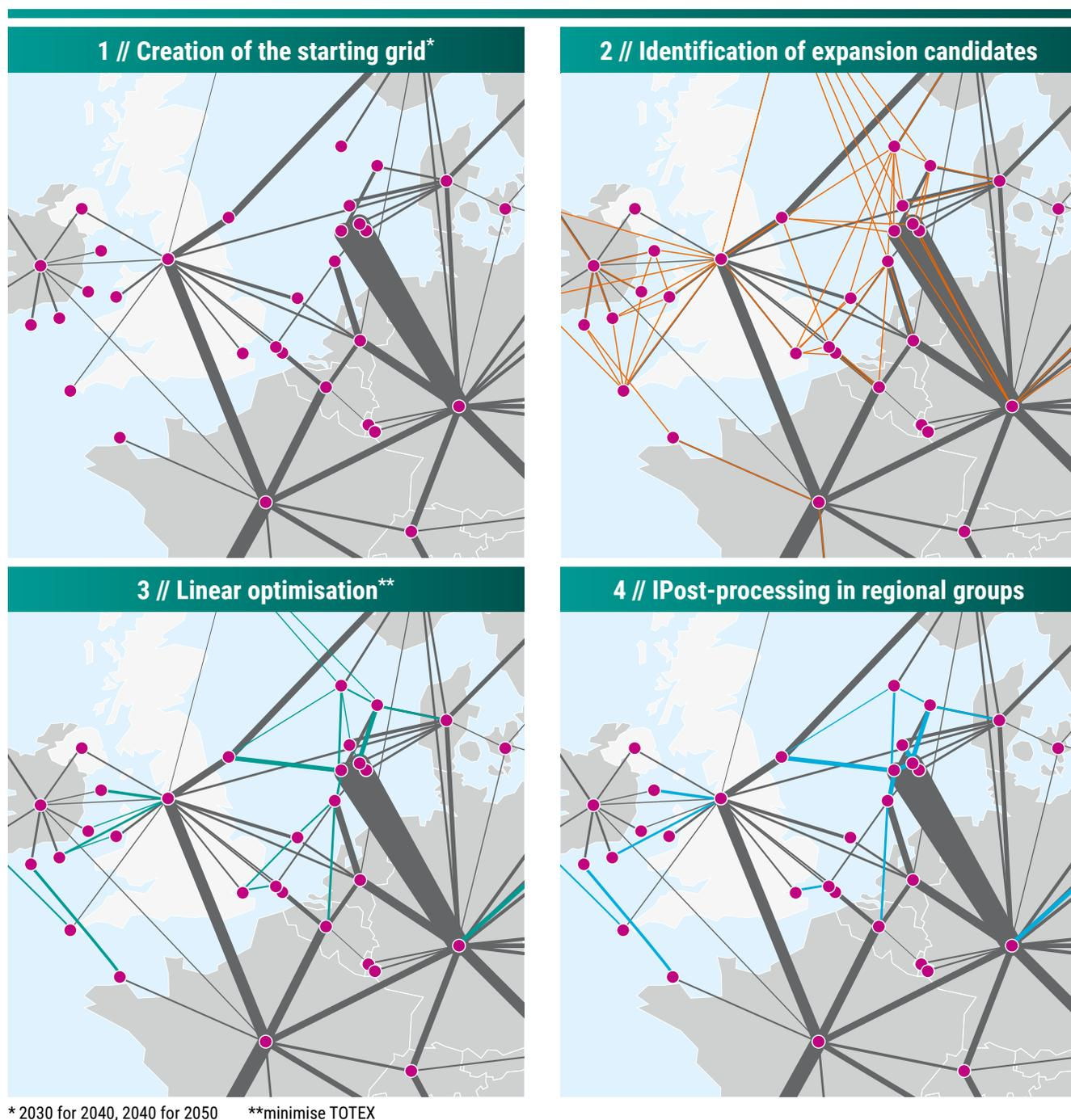
Figure 5 – Schematic Visualisation of the ONDP expansion loops.
