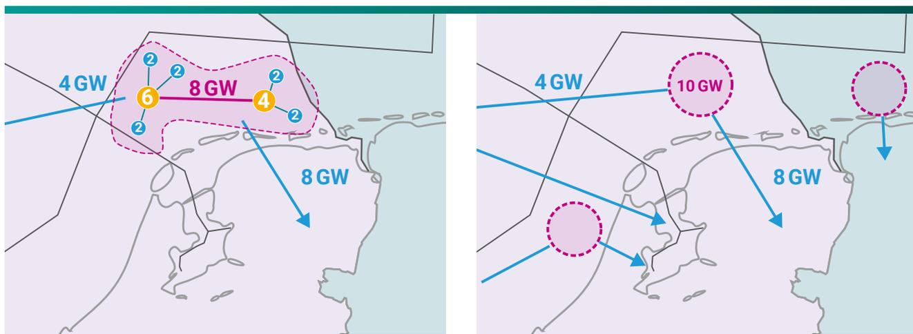
Figure 9 – Step 1 – Aggregation of offshore RES Clusters into nodes in the model. The ONDP will give the details about the distribution of the generation capacities and transmission infrastructure inside the modelling nodes in step 3.
