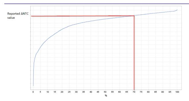
Figure 6: Duration curve of  $\Delta$ NTC in one direction (blue) with 70<sup>th</sup> percentile (red): the reported  $\Delta$ NTC at the 70<sup>th</sup> percentile needs to be reached at least 30% of the time –to the right of the red line.
