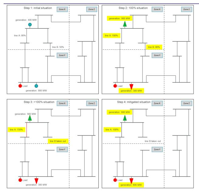
Figure 11: Qualitative example to illustrate the single steps, as described in the example above. It should be noted that the real physical flow will also have a component across the boundary between zones X-Z and Z-Y.
