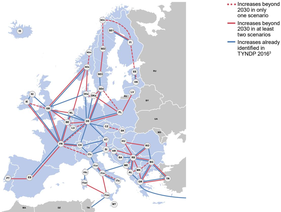
Figure 3: Justification of increases from ST 2040 on top of confirmed increases from previous TYNDP
