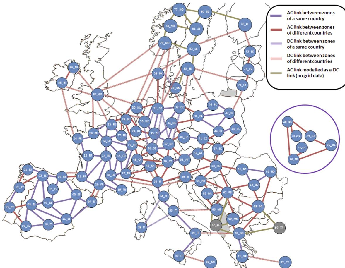
The process leads to a simplified network illustrated in Figure 2, where all substations of a given area are merged in an equivalent node – a “zone” – and all links
