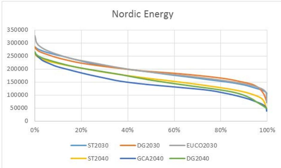
Figure 1 -Energy duration curve In the Nordic Synchronous Area
