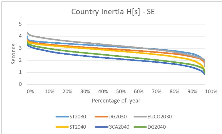
Figure 2 – Inertia duration curve in Sweden
