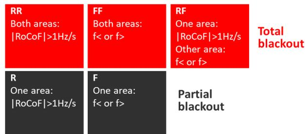
Figure 2 – Conditions for blackout due to RoCoF higher in absolute value to 1 Hz/s or by a frequency exceeding the frequency band of 47.5–51.5 Hz
