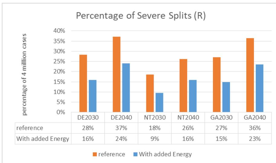
Figure 10 – percentage of severe splits with added energy sized such to reduce *Global Severe Splits* to zero for the NT 2030 scenario.
