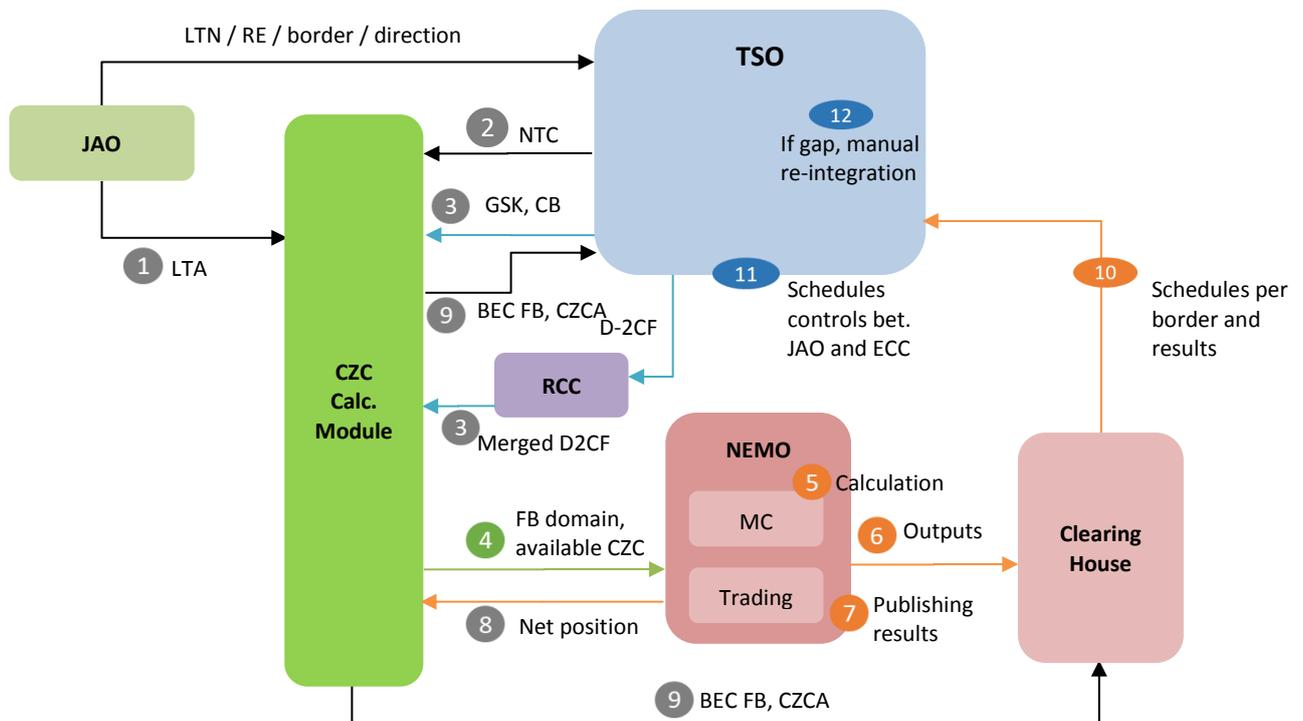
FIGURE 3: MAIN FUNCTIONS OF THE SINGLE DAY-AHEAD COUPLING
