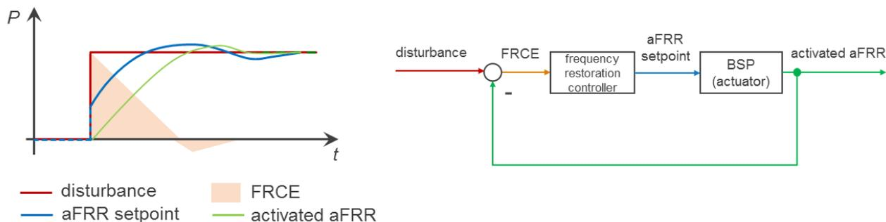
Figure 17: Example for closed control loops
