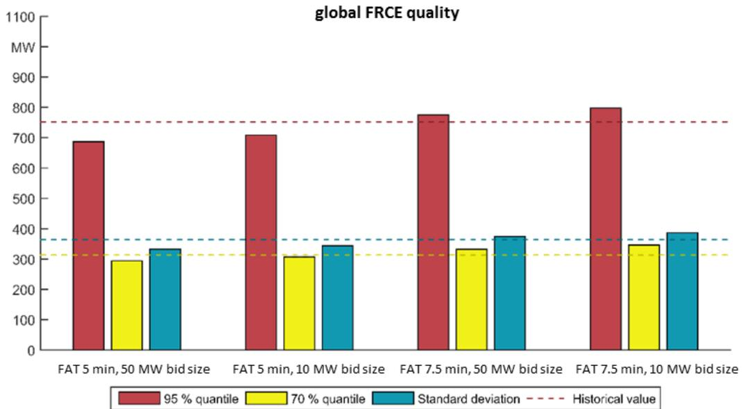
Figure 5: Simulation results for the global FRCE quality
