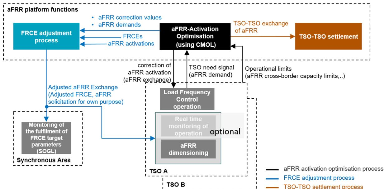
Figure 16: Activation optimisation function with control demand model
