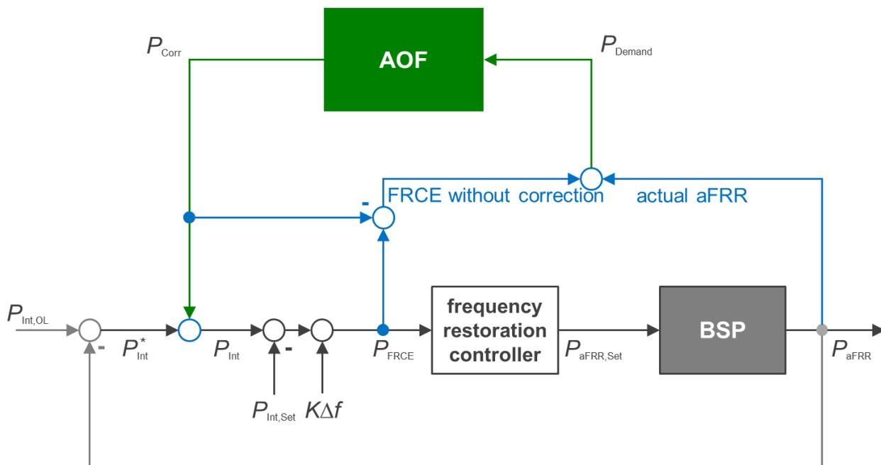
Figure 20: Scheme of the control demand model
