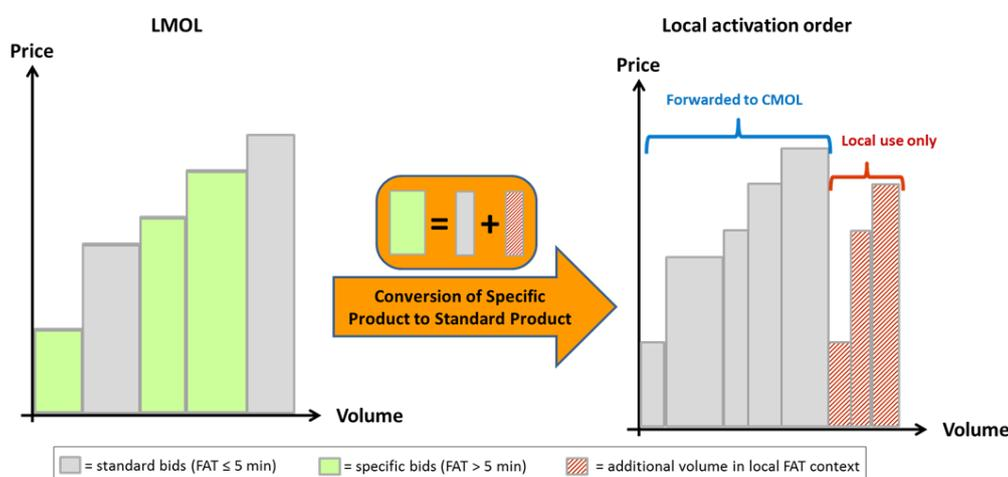
Figure 8: Local implementation of option 1, with conversion of specific products
