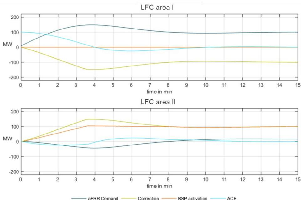
Figure 24: Example for an exchange of aFRR from LFC area II towards LFC area I with the control request model
