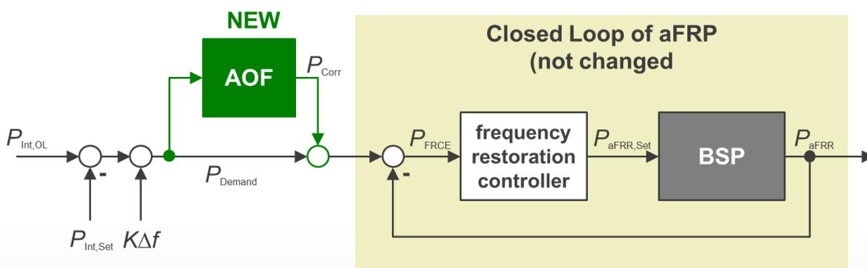
Figure 21: Structural proof of stability for control demand method
