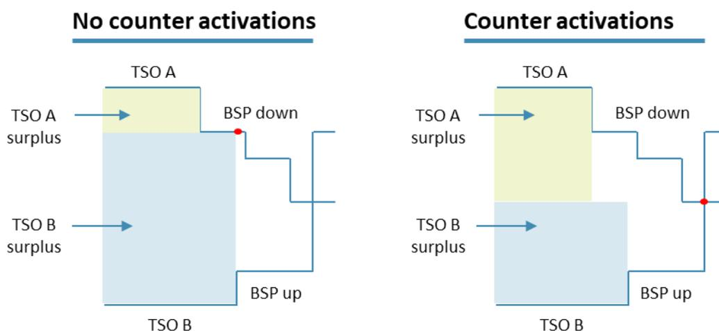
Figure 32: Effect of counter activations on distribution of TSO surplus
