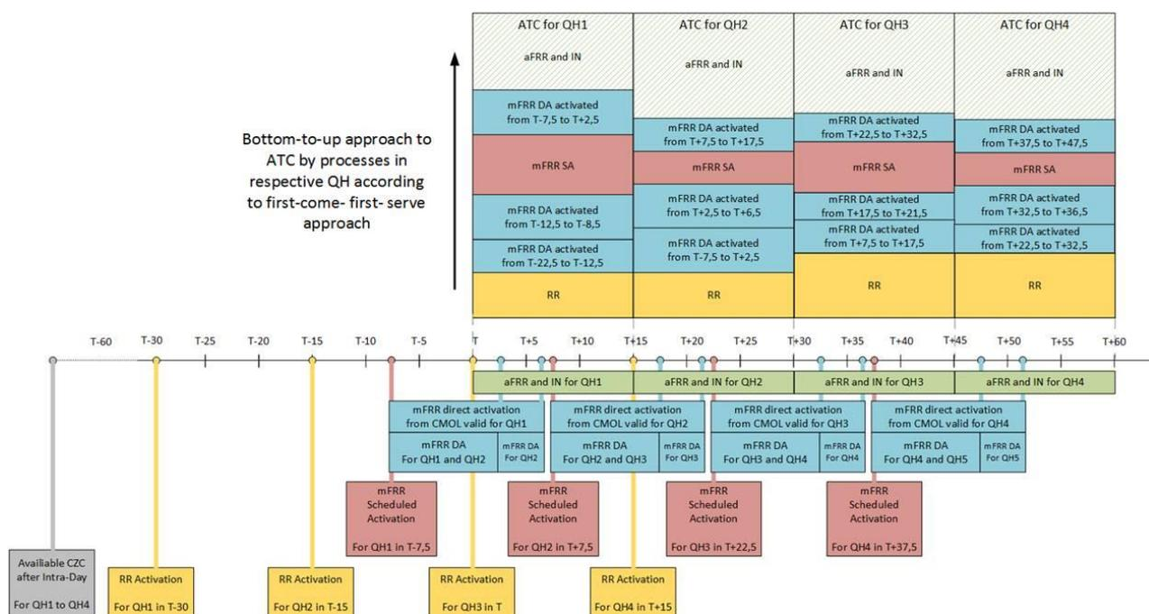
Figure 39: Timeline of activation in platforms with first-come-first-serve approach to capacities
