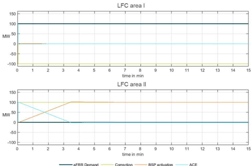
Figure 23: Example for an exchange of aFRR from LFC area II towards LFC area I with the control demand model
