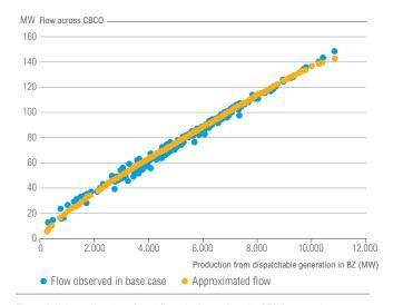
Figure 6.6: Approximation of load flows in the merit-order PTDF approach (for an illustrative line); Note: 'Generation' refers to dispatchable generation only, i. e. excluding variable RES
