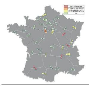
Figure 4.8: Projected physical flows in France in 2030 (MWh/h)
