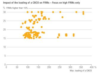
Figure 6.8: Correlation between loading of a CBCO and its FRM
