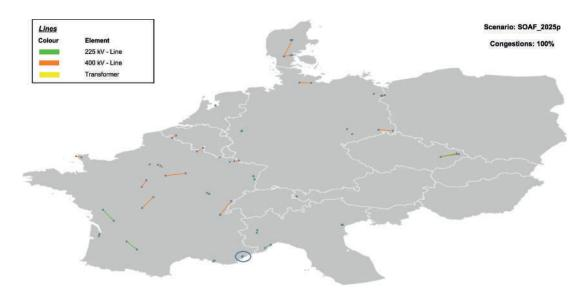
Figure 4.29: All N-0 grid constraints per voltage level in the SOAF 2025 worst case scenario – based on the assumption of an only partial implementation of the planned network extensions
