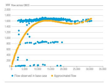
Figure 6.7: Deviations between actual and approximatised load flows (for an illustrative line)
