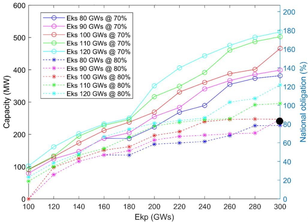
Figure 3 Estimated FCR-D capacity in Finland, based on installed capacity and distribution of water time constant, as a function of system kinetic energy. Black circle fulfils dimensioning requirements [3].
