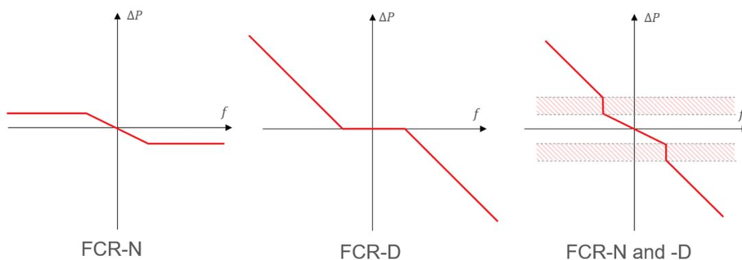
Figure 5 Steady state relationship between power change,  $\Delta P$ , and frequency,  $f$ , of a conventional regulator (2) with switching of droop at 49.9/50.1 Hz ( $\text{droop}_{\text{FCR-N}} > \text{droop}_{\text{FCR-D}}$ ).
