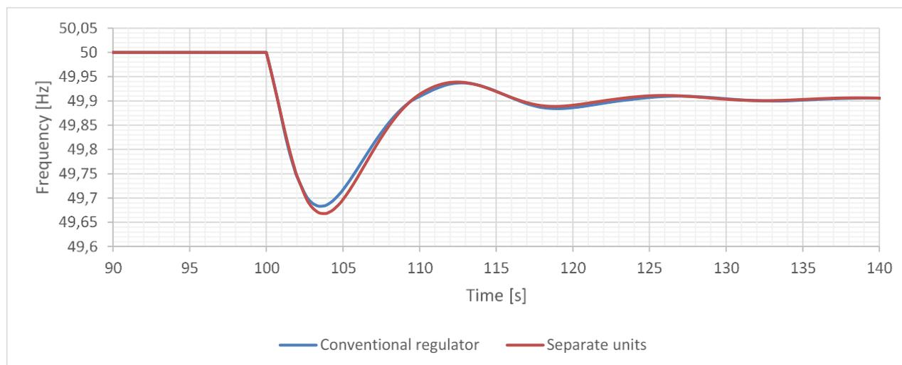
Figure 6 Comparison of the dynamic system behaviour after a 600 MW unit trip when using different units for supplying the FCR services (brown) and when using FCR services from the same units using,  $K_{P, FCR-N}=4.4$  and  $K_{P, FCR-D}=10.4$ .
