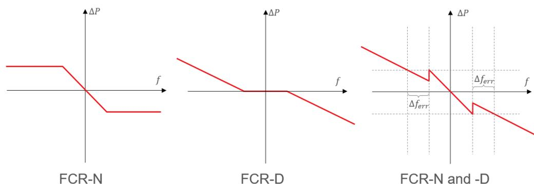
Figure 4 Steady state relationship between power change,  $\Delta P$ , and frequency,  $f$ , of a conventional governor (2) with switching of droop at 49.9/50.1 Hz ( $\text{droop}_{\text{FCR-N}} < \text{droop}_{\text{FCR-D}}$ )
