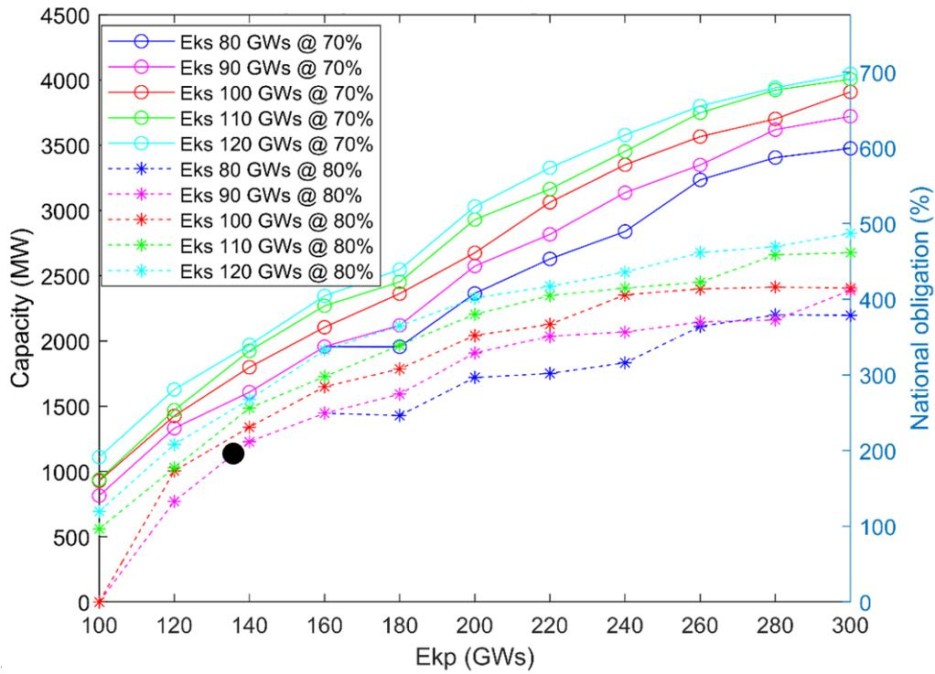
Figure 2 Estimated FCR-D capacity in Sweden, based on installed capacity and distribution of water time constant, as a function of system kinetic energy. Black circle fulfils dimensioning requirements [3].
