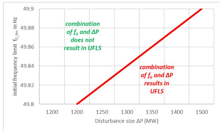
Figure 14: Example of  $f_{0\_lim}$  equation (1).
