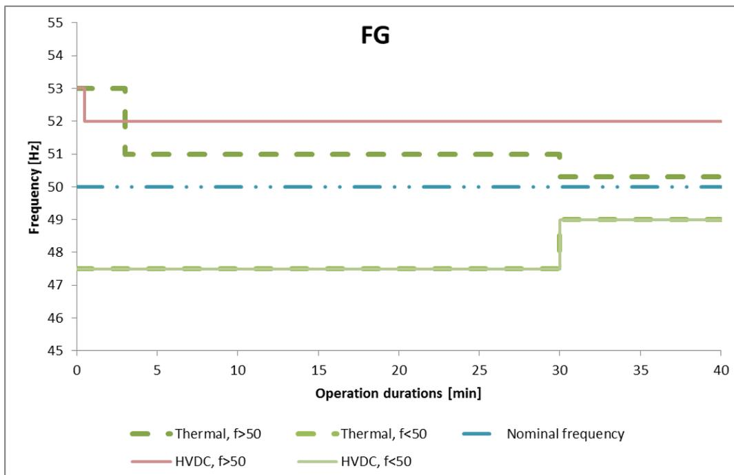
Figure 36 Frequency minimum levels, time scale 0-40 minutes, Finland.
