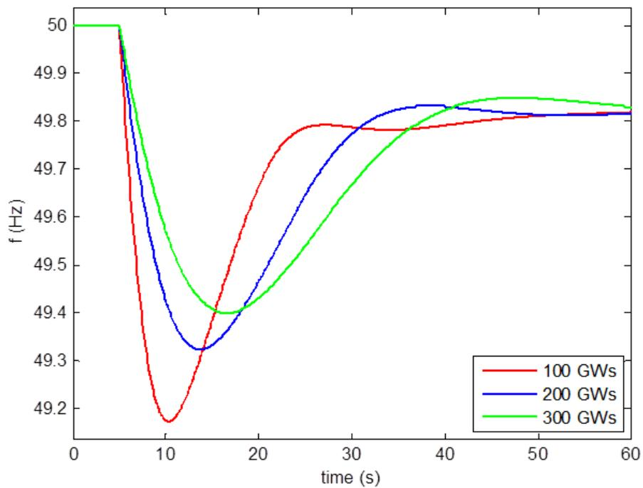
Figure 23 Simulated response for frequency response when losing a large generating unit, as a function of different system inertia levels.
