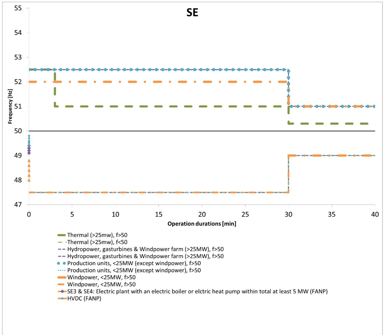
Figure 39 Frequency minimum levels, time scale 0-40 minutes, Sweden.
