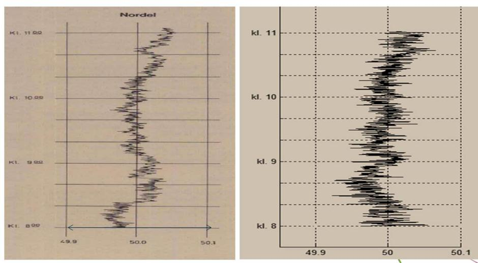
Figure 2 Oscillations have increased in 40 years ([35] and 2012 measurement values from ENDK Scada system)
