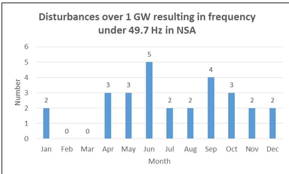
Figure 27 Monthly distribution of frequency drops deeper than 49.7 Hz in years 2003-2013.
