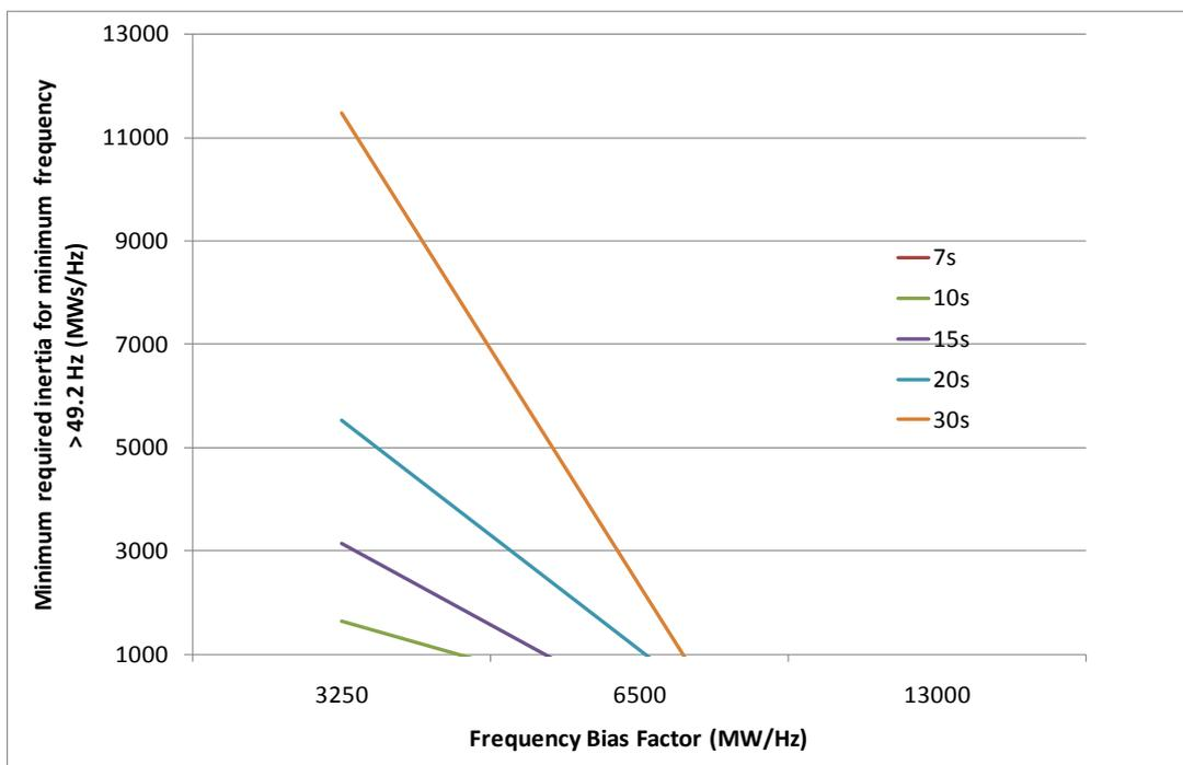
Figure 17 Minimum inertia in the system that is required for keeping the minimum frequency above 49.2 Hz for several values of the Frequency Bias Factor for different system time constants of the FCR-D [36]. See also footnote 17.
