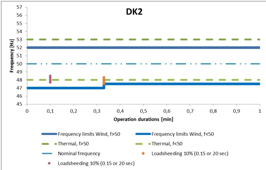
Figure 37 Frequency minimum levels, time scale 0-1 minutes, Denmark (DK2).
