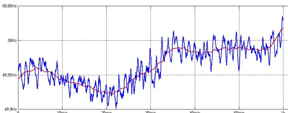
Figure 18 Original frequency measurement (blue) and a filtered frequency (eliminating the 60 s oscillation) (red) [41]
