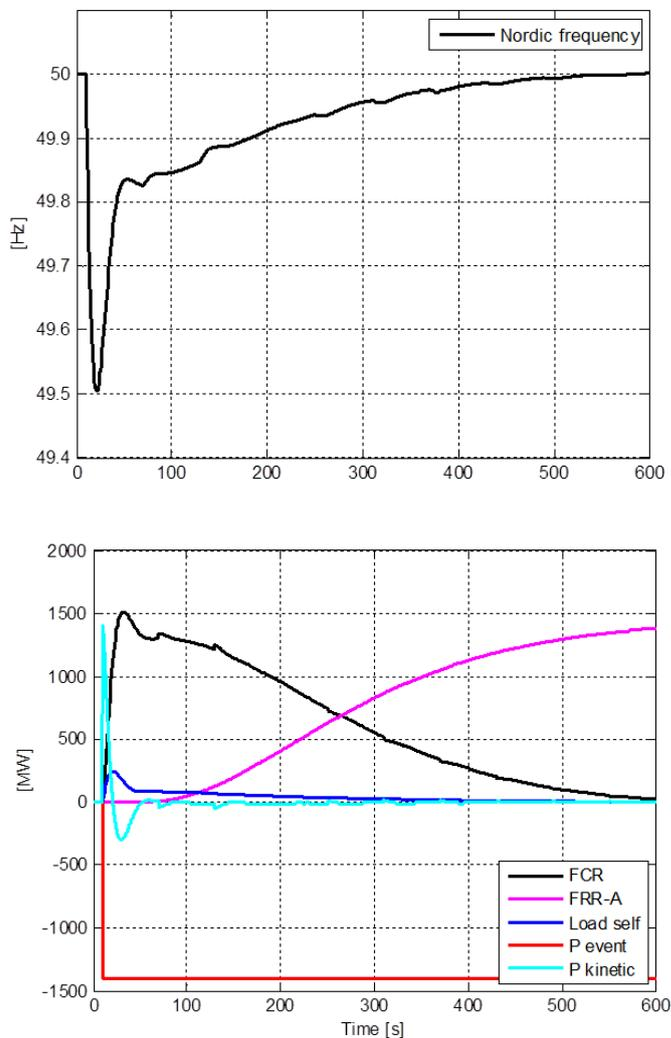
Figure 14 Response of Inertia, FCR and FRR-A after an outage.
