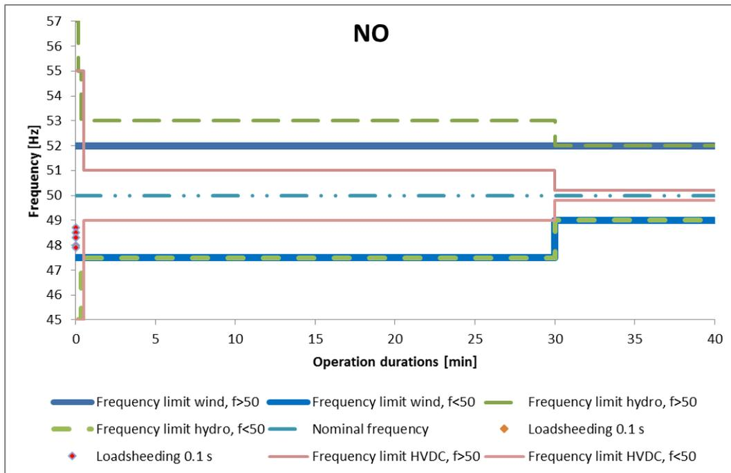
Figure 35 Frequency minimum levels, time scale 0-40 minutes, Norway.
