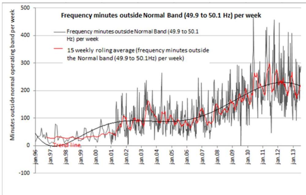
Figure 1 Frequency quality trend 1996-2013 based on weekly minutes outside the band. A change in data characteristics in January 2001 due to going from monthly to weekly average values.
