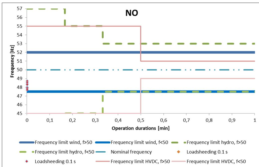
Figure 34 Frequency minimum levels, time scale 0-1 minutes, Norway.
