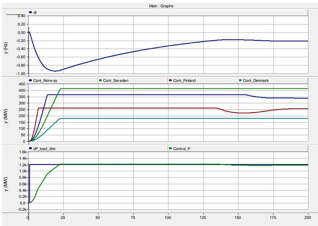
Figure 30 Responses in case of 1200 MW loss of production. From top: Frequency deviation/ Reserve power responses of each TSO / Power trip and total control power response. Inertia 10000MWs/Hz, FBF = 5230 MW/Hz, Control with present time constants according RAR report. See footnote 23.
