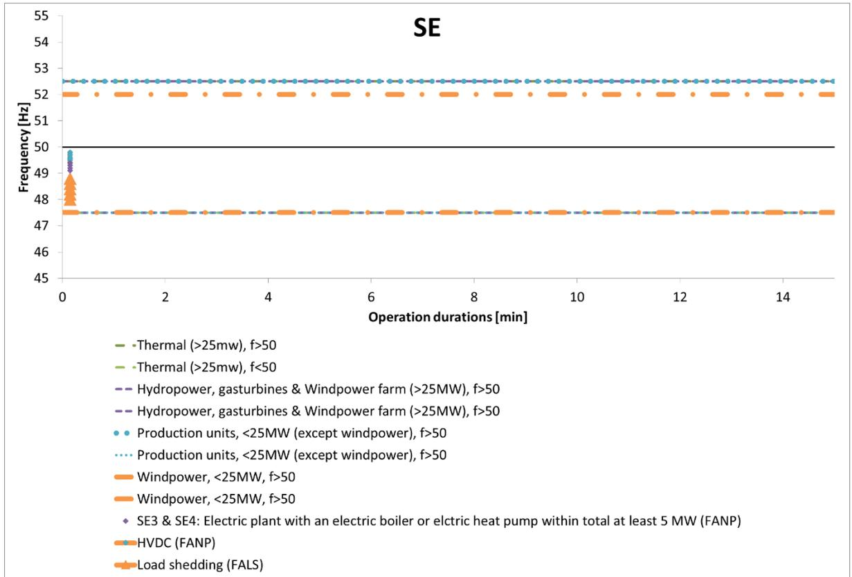
Figure 40 Frequency minimum levels, time scale 0-14 minutes, Sweden.
