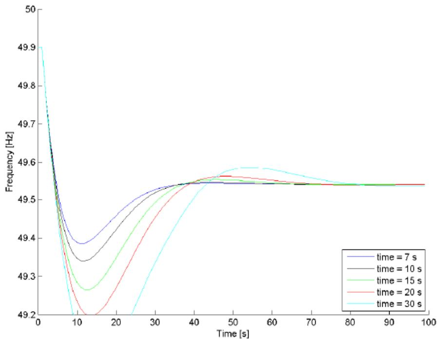
Figure 24 Relations between speed of FCR and frequency network characteristic for steady state frequency of 49.5 Hz (frequency deviation after outage is 400 mHz). Loss of production is 1300 MW, FBF 3250 MW/Hz, Inertia 250 GWs [36].
