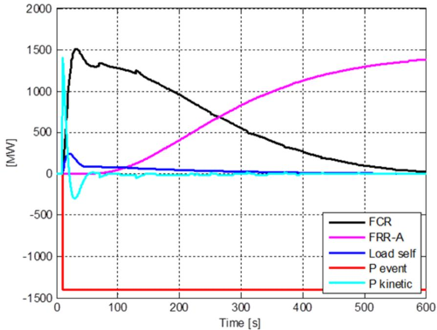
Figure 10 An illustration of calculated power contributions after tripping 1400 MW production. Note: only illustrative figure (not measured response from real disturbance). RAR-model used for simulation [36].
