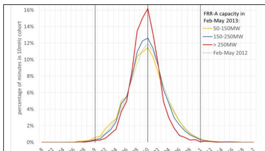
Figure 5 Distribution of frequency, separate for three levels of FRR-A during the test period from February to March 2013. [42]
