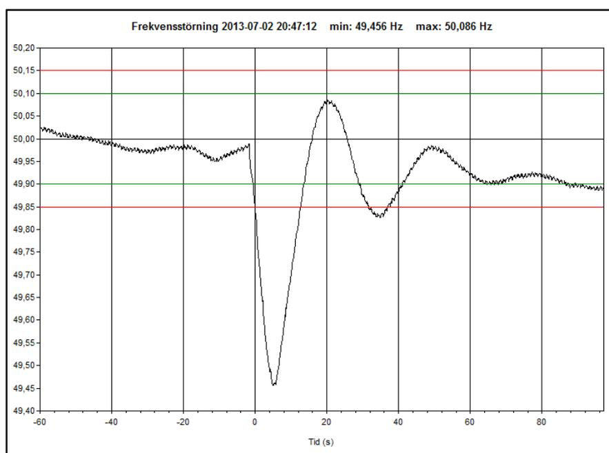
Figure 4 Typical frequency profile after forced outage of a large production unit (nuclear power plant).
