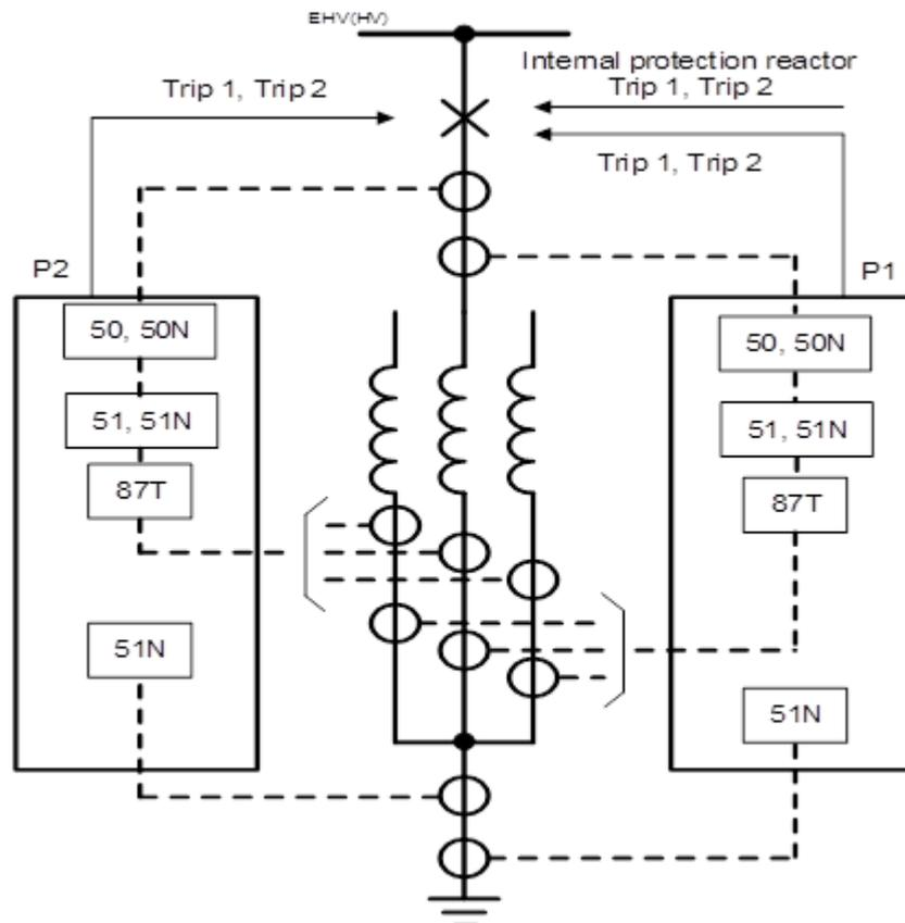
Figure I Example of a protection system proposed for a shunt reactor (indicative)
