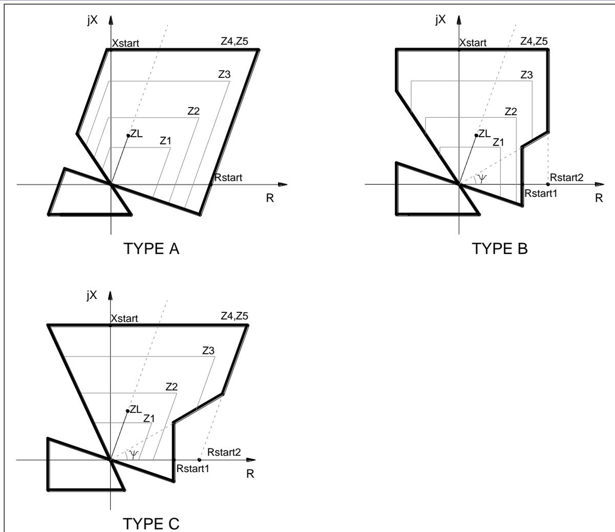
Figure: Main features of starting distance protection
