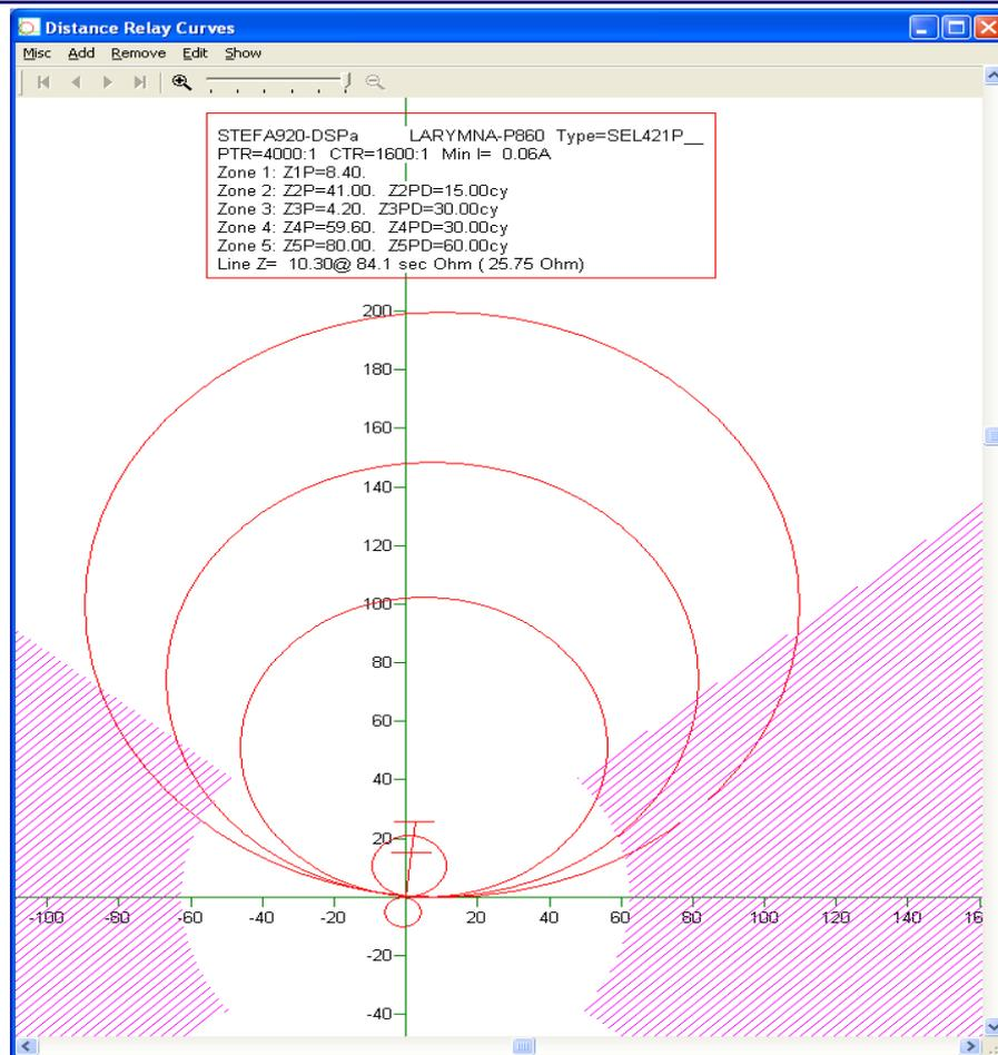
Figure 2: Load encroachment characteristic
