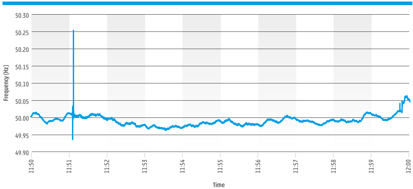
Figure 3.20: WAMS frequency measurement at the HRA substation in the V412 line bay from 11:50 to 12:00
