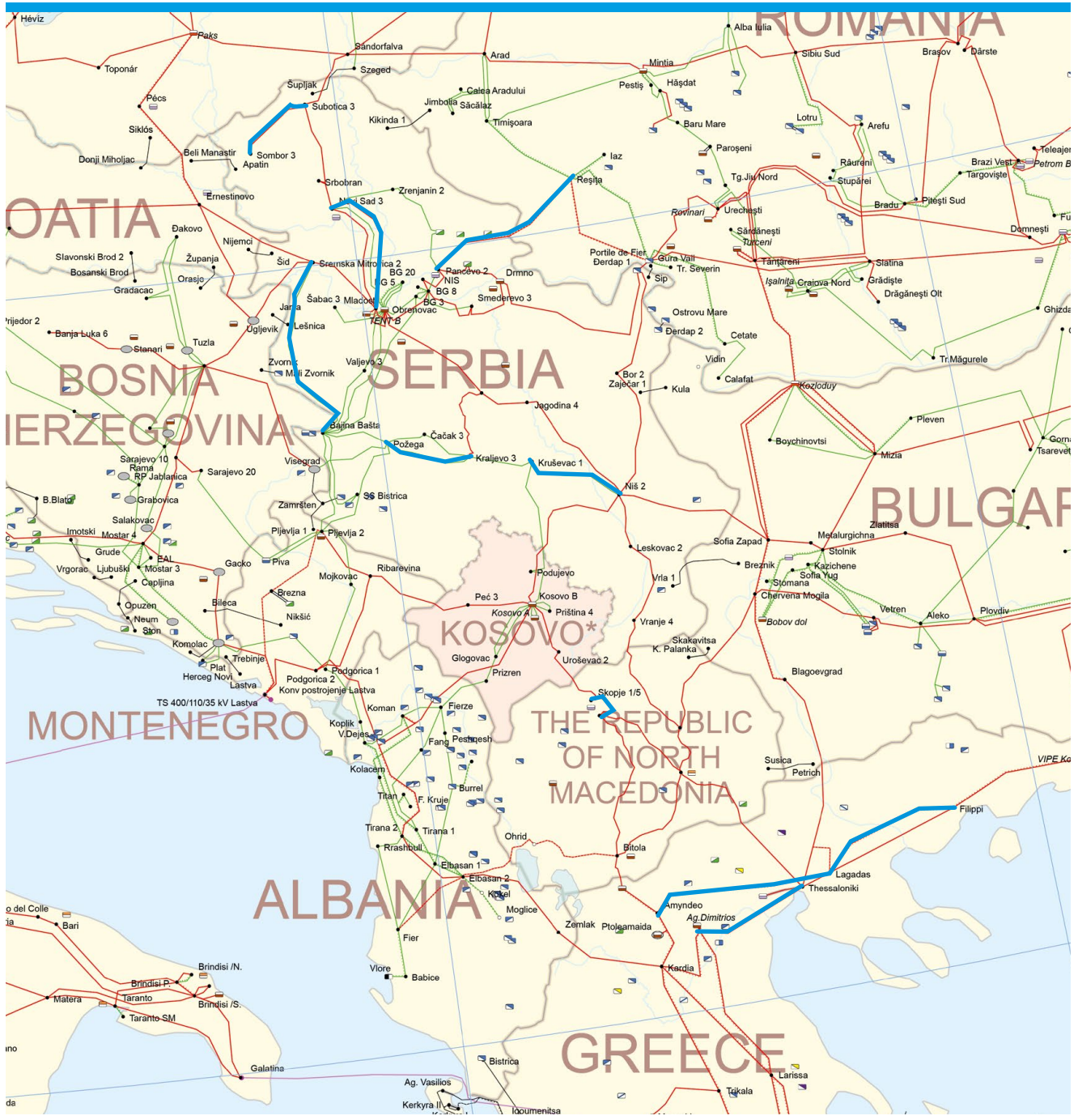
Figure 7.27: Disconnected OHLs in the SEE region for voltage control purposes.
