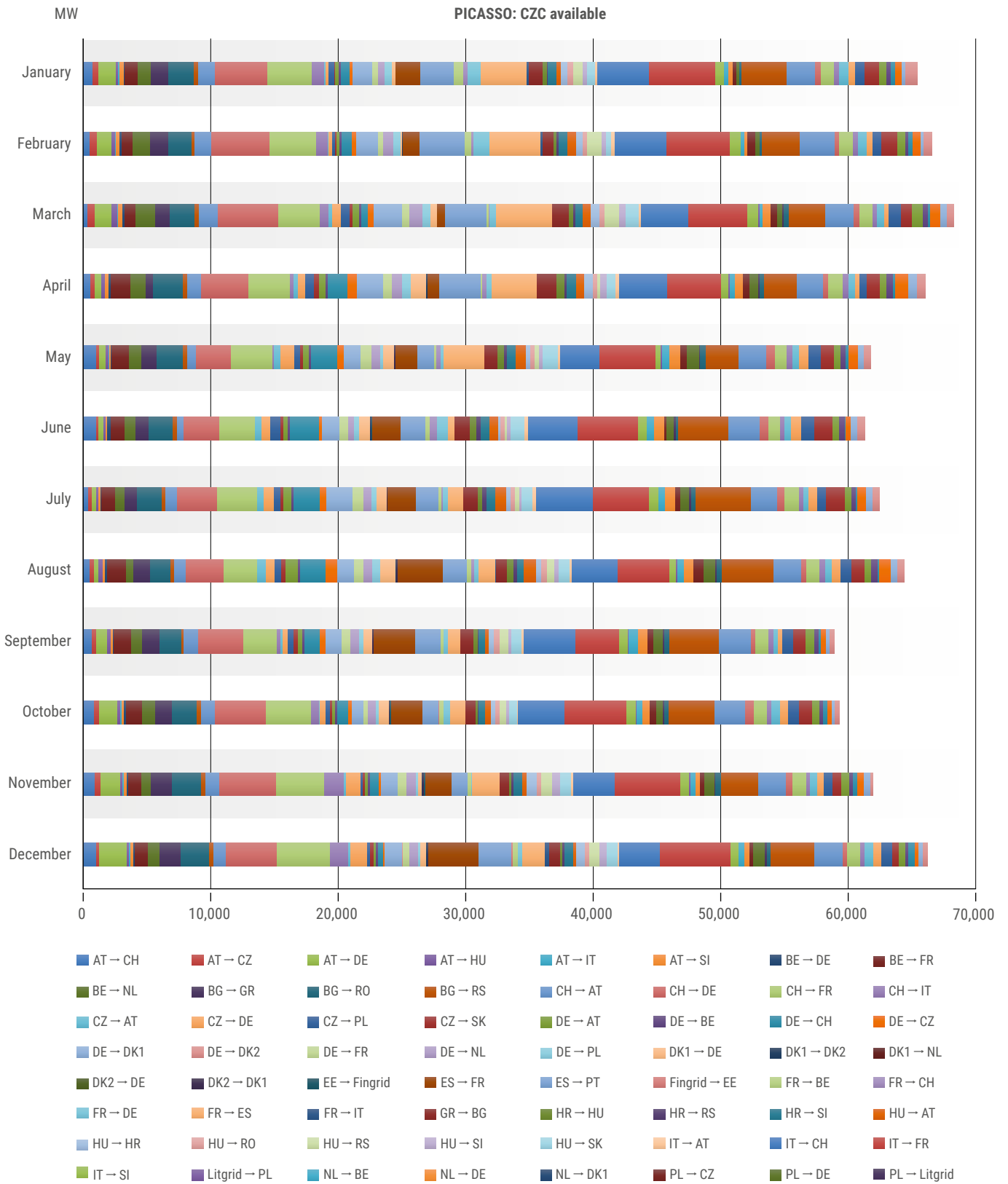
Figure 107: KPI 6.4.6: aFRR platform: monthly average value of the available CZC per BZB and direction (MW/MTU)
