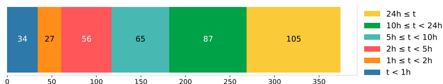
Figure 10.33: Number of ICS violations grouped by duration in 2025 for Ukrenergo.
