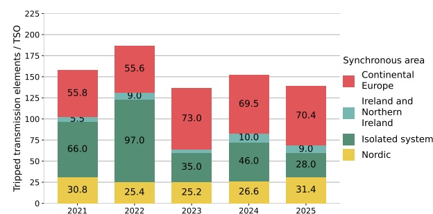
Figure 5.1: Operational security indicator OS-A from 2021–2025. It is calculated by adding up the number of tripped transmission system elements reported for all scale 0–3 incidents, and dividing by the number of TSOs in the synchronous area.
