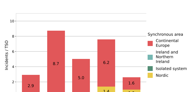
Figure 5.7: Operational security indicator OS-E2 from 2021–2025. It is calculated by counting the number RRC0-, RRC1- and RRC2-incidents and the number of all other scale 0–3 incidents if a reduction of reserve capacity is reported, and dividing by the number of TSOs in the synchronous area.
