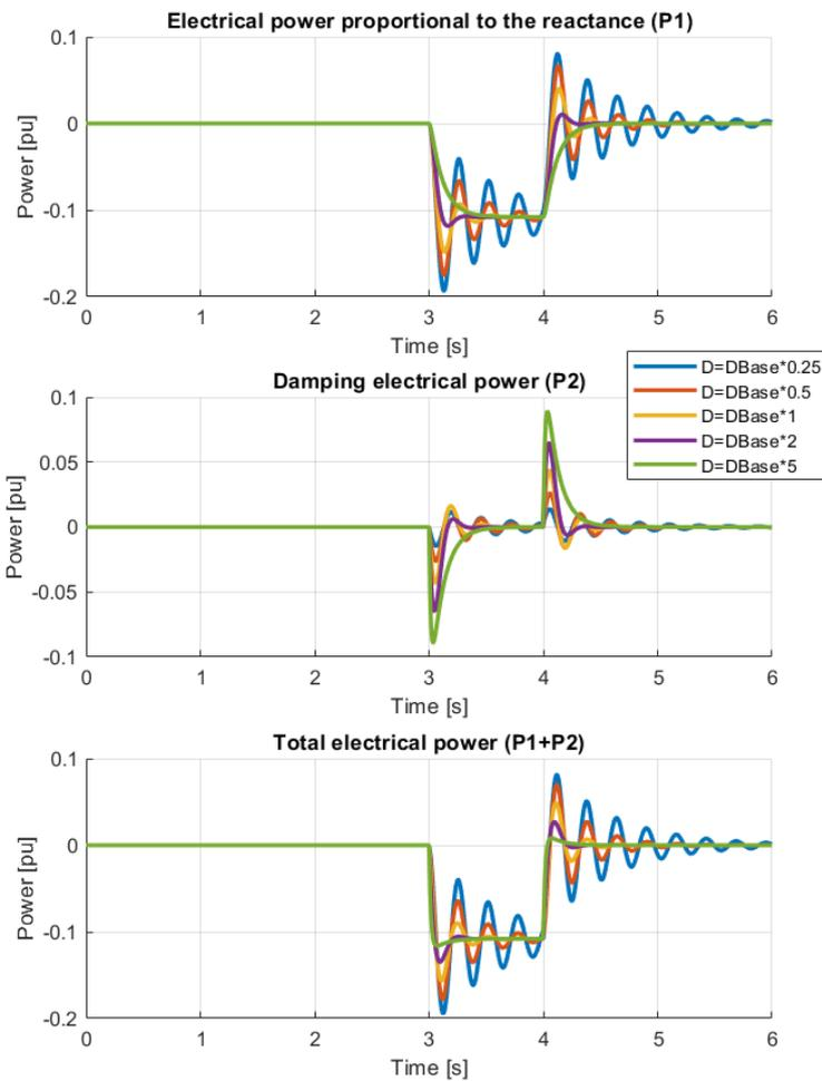
Figure 14. Comparison of real and simulated powers during an under frequency event as a function of the level of damping.
