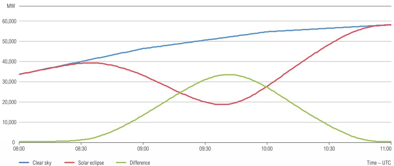
Figure 2: Comparison of expected feed-in from solar on 20 March during clear sky conditions with and without solar eclipse.
