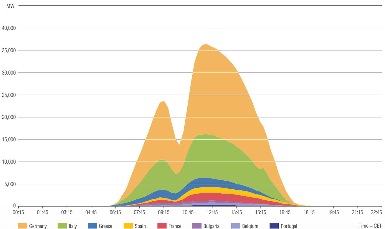
Figure 5: Aggregated PV feed-in from a subset of European TSOs
