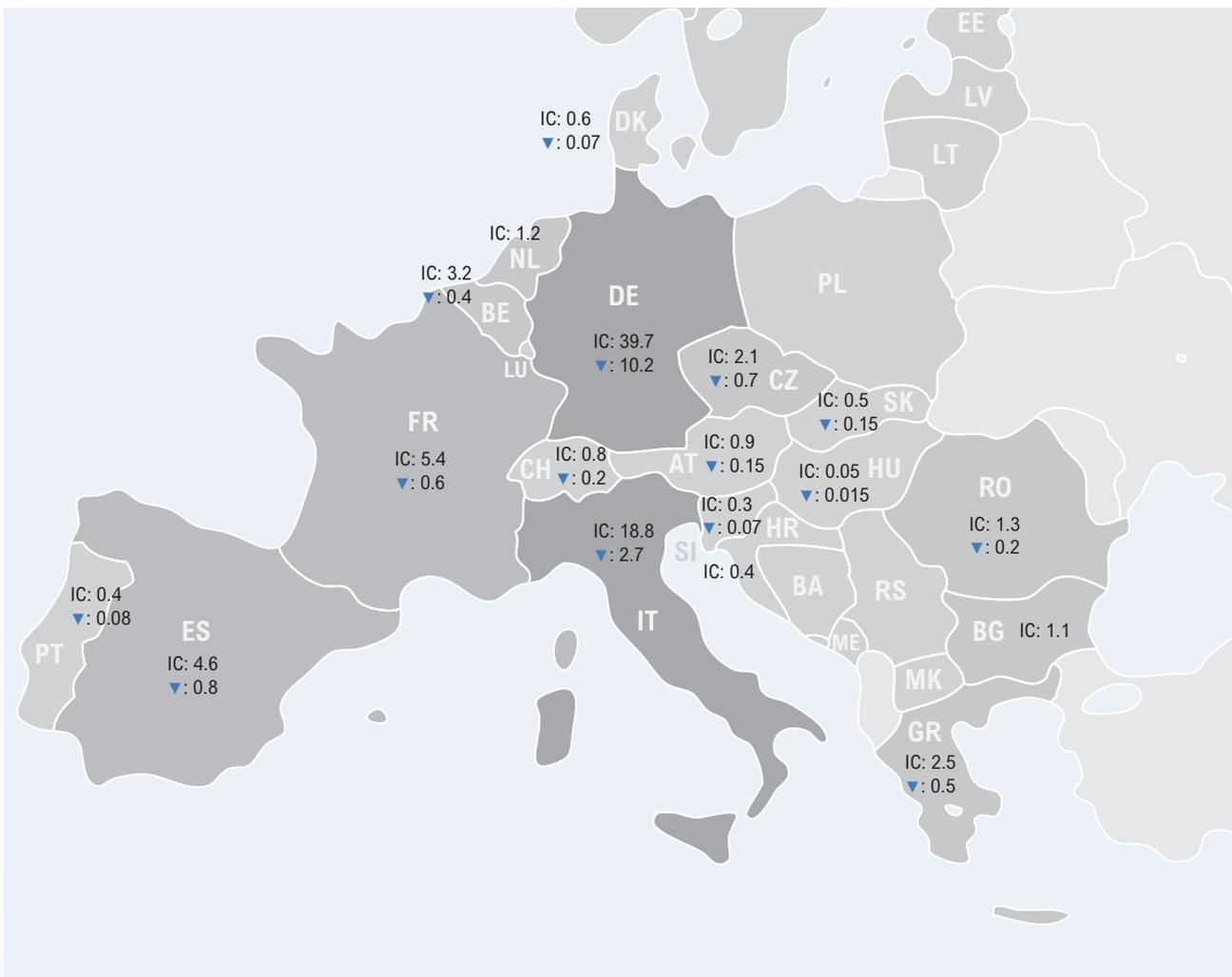
Figure 3: Continental Europe installed PV capacity in GW (IC) and estimated eclipse impact (▼ x GW drop)
