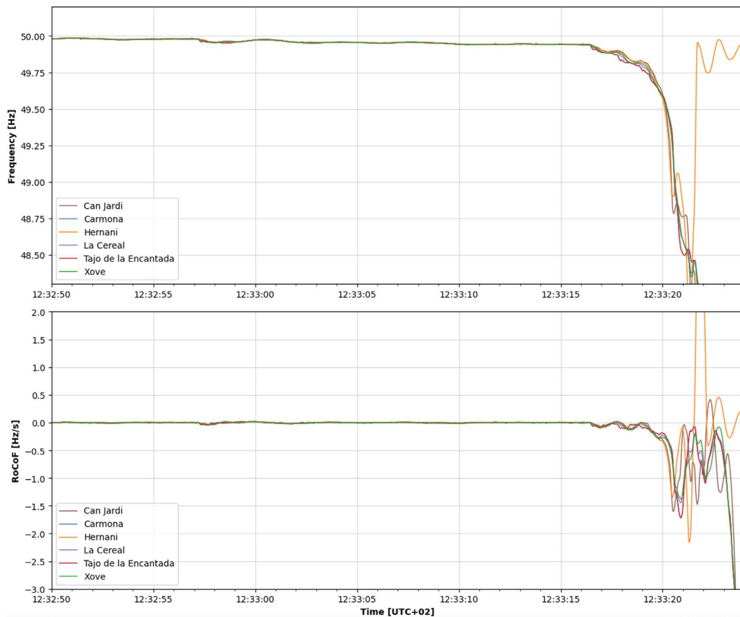
Figure 3-8: Frequency and RoCoF in the Spanish power system during the incident
