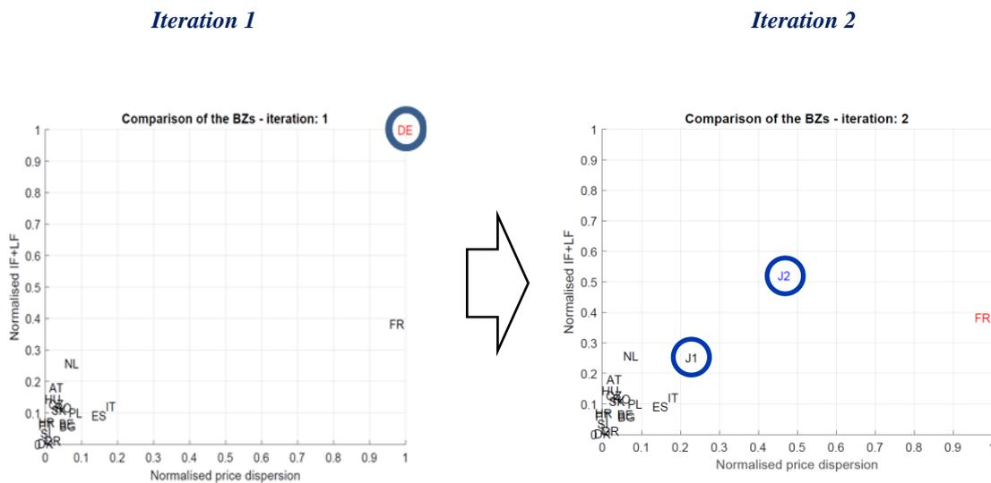
*Note: For simplicity and illustration purposes, only iterations 1 and 2 are shown. J1 and J2 refer to the newly identified BZs following a split of Germany into two BZs as a result of iteration 1. The example illustrates how a BZ change potentially improves the performance in terms of economic efficiency (decreasing price dispersion within BZs) and cross-zonal capacity (decreasing the amount of loop flows and internal flows on network elements that are relevant for capacity calculation).*
