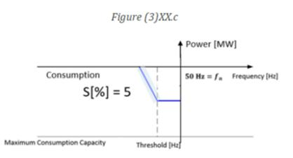
Pref is the actual active power at the moment the LFSM-UC threshold is reached.
