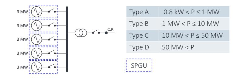
Each unit has its own breaker and can therefore be started, stopped, connected and disconnected/tripped **independently** from the others.
