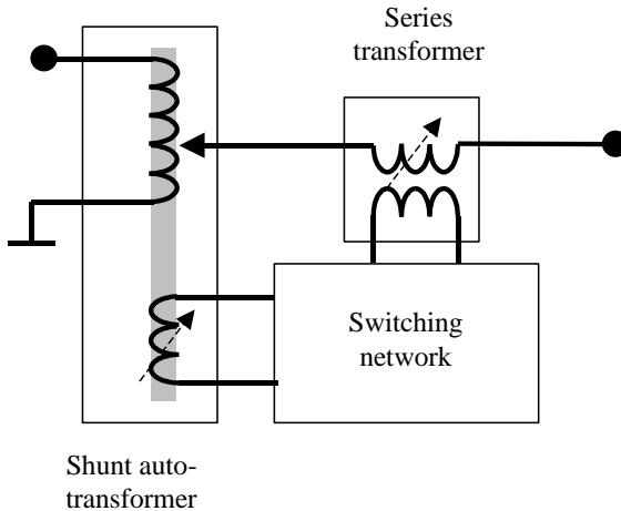
The phase shift regulation may be on the shunt or on the series transformer
